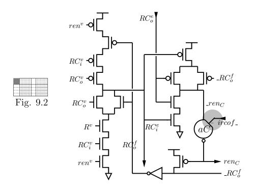
Figure 9.19: PCEVHB WAD nested read handshake control circuit. The shaded circuit is a modification introduced by WAD nesting.
