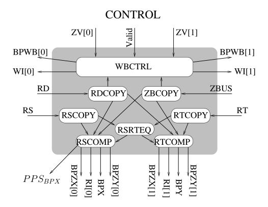
Figure 7.3: Schematic of Control decomposition for port priority select
