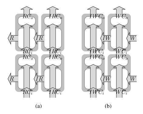
Figure 9.1: Block diagram of vertically pipelined, and nested read and write processes.
