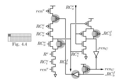
Figure 5.13: Single port of a width-adaptive read handshake control, PCEVHB reshuffling (resets not shown). Shaded circuits are modifications introduced by WAD.
