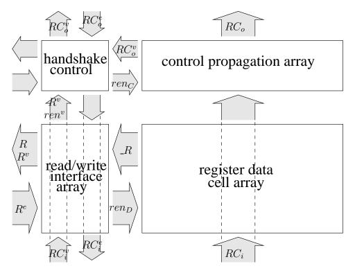
Figure 4.5: Floor decomposition of a read port block, shown with channel signals and some internal signals at component boundaries
