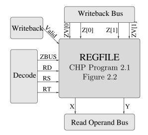
Figure 2.1: Register file's channel interface with its environment
