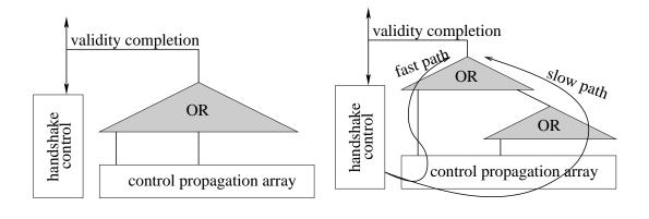
(a) Balanced completion trees (b) Unbalanced completion trees
