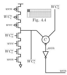
Figure 4.17: Write handshake control for full-buffered unconditional control propagation. (resets are not shown)
