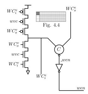
Figure 4.18: Write handshake control for half-buffered unconditional control propagation. (resets are not shown)
