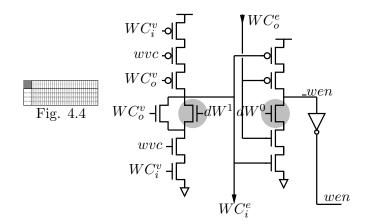
Figure 5.17: Single port of a width-adaptive write handshake control, with conditional write-enable, PCEVHB reshuffling (resets not shown). Shaded circuits are modifications introduced by WAD.
