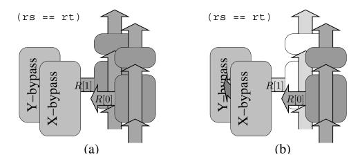
Figure 7.1: a) A traditional multi-ported register file may retrieve the same register through different ports, whereas b) a PPS implementation may reduce energy by suppressing redundant read accesses to the core.
