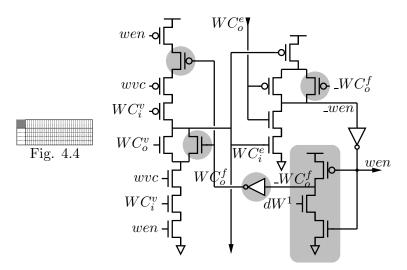
Figure 5.14: Single port of a width-adaptive write handshake control, with unconditional write-enable, PCEVFB reshuffling (resets not shown). Shaded circuits are modifications introduced by WAD.
