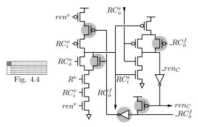
Figure 5.12: Single port of a width-adaptive read handshake control, PCEVFB reshuffling (resets not shown). Shaded circuits are modifications introduced by WAD.
