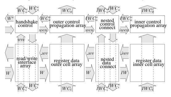
Figure 9.4: Floor decomposition of a data-nested core write port
