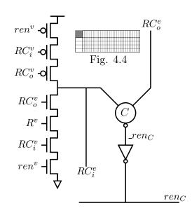
Figure 4.15: Read handshake control for full-buffered unconditional control propagation. (resets are not shown)
