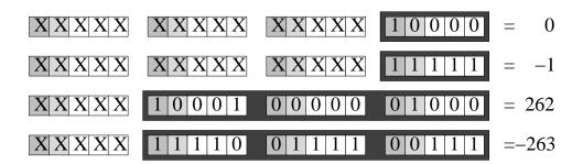
Figure 5.2: Examples of width-adaptive representation of integers. The delimiter bits are darkly shaded, and the MSBs are lightly shaded. X's represent 'don't cares.' Only darkly bordered bits are communicated.
