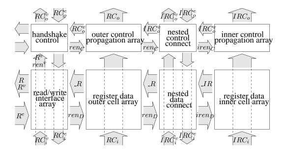
Figure 9.3: Floor decomposition of a data-nested core read port
