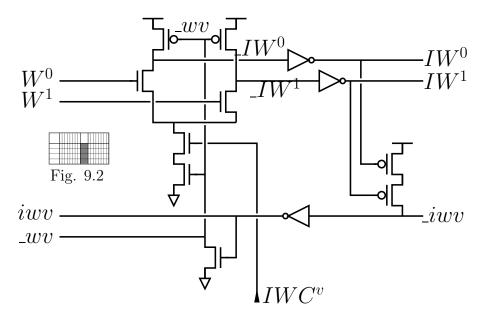
Figure 9.16: The interconnect circuit between inner and outer register partitions for a single nested write port
