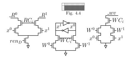
Figure 4.11: QDI Register core cell. Only one read and one write port are shown.
