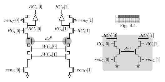
Figure 5.10: Width-adaptive pipeline-locked read control propagation, two ports shown. Shaded circuits are modifications introduced by WAD.
