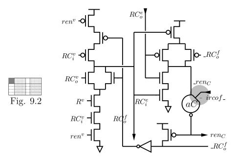
Figure 9.18: PCEVFB WAD nested read handshake control circuit. The shaded circuit is a modification introduced by WAD nesting.
