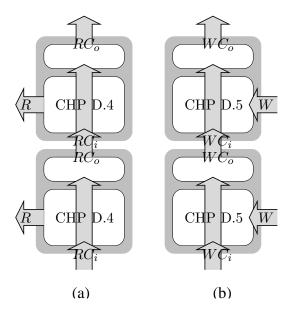
Figure 3.5: Pipelined core process blocks for a) reading and b) writing
