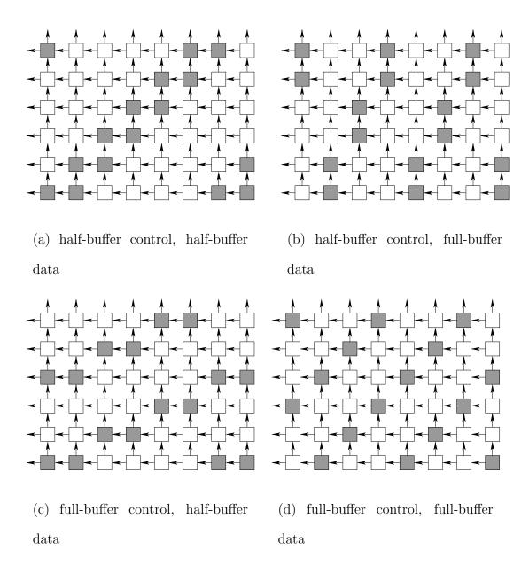
Figure 4.3: Examples of two-dimensional pipelining. The control pipeline is vertical, and the data pipeline is horizontal. Tokens are represented by diagonal bands of colored rectangles.
