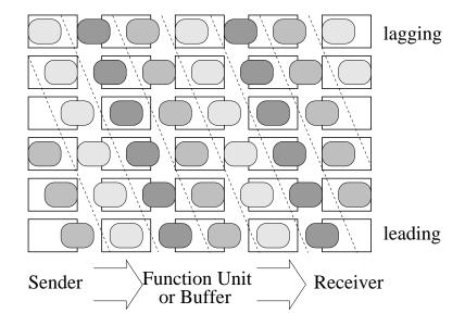
Figure 3.4: Snapshot of vertically pipelined, block-skewed datapath communication. Like-shaded rectangles correspond to the same logical token. Control to functional units are issued from the bottom, and propagated to the upper blocks, thus the lower blocks will *lead* the upper blocks.
