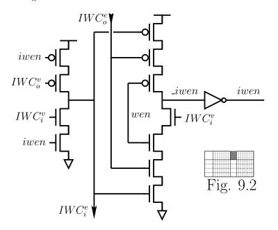
Figure 9.22: The control interconnect circuit between inner and outer partitions' control propagation arrays for a non-WAD nested write port
