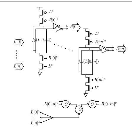
Figure 1.4: Abstract PCHB circuit template for a function with n inputs and m output channels.
