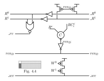
Figure 4.14: Read and write data interface for a single port of a bit line (resets are not shown)
