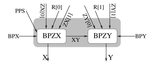
Figure 7.2: Modified read bypass decomposition for Port Priority Selection
