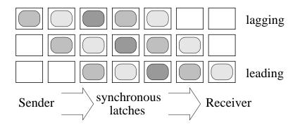
Figure 3.3: Synchronous parallel skewed vertical pipeline operation
