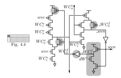
Figure 5.15: Single port of a width-adaptive write handshake control, with unconditional write-enable, PCEVHB reshuffling (resets not shown). Shaded circuits are modifications introduced by WAD.
