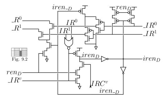
Figure 9.15: The interconnect circuit between inner and outer register partitions for a single nested read port
