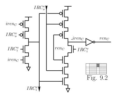
Figure 9.20: The control interconnect circuit between the inner and outer partitions' control propagation arrays for a non-WAD nested read port
