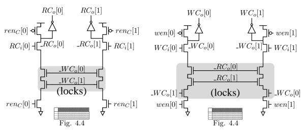
Figure 4.12: Pipeline-locked read control propagation, shown for two ports.
