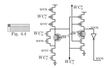
Figure 5.16: Single port of a width-adaptive write handshake control, with conditional write-enable, PCEVFB reshuffling (resets not shown). Shaded circuits are modifications introduced by WAD.
