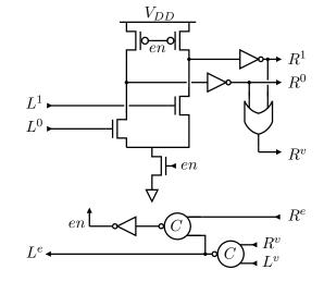
Figure 4.1: Precharge enable-valid fullbuffer (PCEVFB) template
