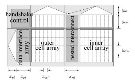
Figure 9.2: Floorplan of a nested 4-bit x 16-word pipeline block of the register core, with the outer partition on the left side and the inner partition on the right. New or modified components that arise from nesting are darkly shaded, while all other components corresponding to Figure 4.4 remain unchanged. The WAD, nested floorplan includes one more row of delimiter bit cells in the cell array. The dimensions for the various components are listed in Table 4.1.
