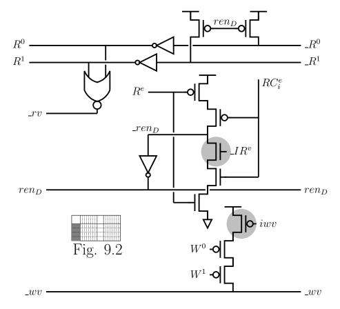
Figure 9.17: The data interface cell adapted to accommodate nested read and write register arrays, shown for a single port. Shaded transistors are modifications introduced by nesting.
