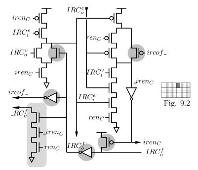
Figure 9.21: The control interconnect circuit between the inner and outer partitions' control propagation arrays for a WAD nested read port. Shaded circuits are modifications introduced by WAD.
