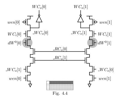
Figure 5.11: Width-adaptive pipeline-locked write control propagation, for unconditional write-enable, two ports shown. Shaded circuits are modifications introduced by WAD.
