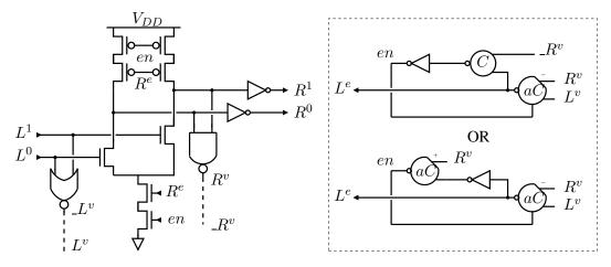
Figure 1.3: Two equivalent implementations of a precharge full-buffer (PCFB) with active-low acknowledgments
