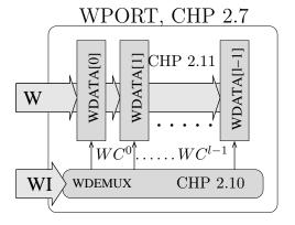
Figure 2.5: Schematic of write port
