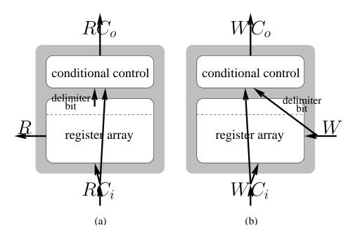
Figure 5.3: Block diagram of a width-adaptive register core a) read port and b) write port
