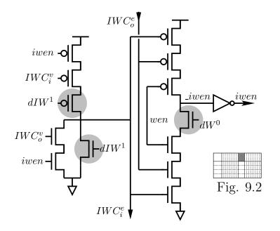
Figure 9.23: The control interconnect circuit between the inner and outer partitions' control propagation arrays for a WAD nested write port with an unconditional outer write-enable. The shaded circuits are modifications introduced by WAD.
