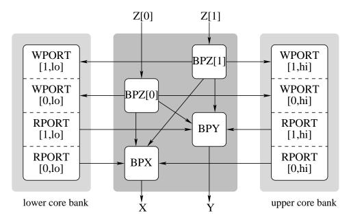
Figure 4.21: Bypass decomposition for dual-banked register core. Control channels are not shown.
