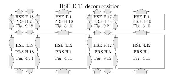
Figure 9.9: Floor decomposition of a PCEVFB WAD nested read port
