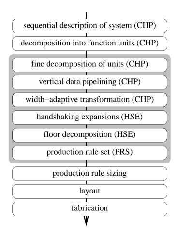
Figure 1.1: Flow diagram of QDI synthesis procedure for an asynchronous system. The design of the register file follows the steps shaded in gray.
