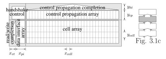
Figure 4.4: Floorplan of a vertically pipelined register core block for reading and writing, from Figure 3.1c
