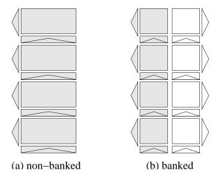
Figure 4.19: Banking the register file is a common method for reducing access energy and delay by reducing the load on bit lines
