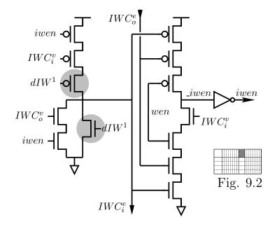
Figure 9.24: The control interconnect circuit between the inner and outer partitions' control propagation arrays for a WAD nested write port with a conditional outer writeenable. The shaded circuits are modifications introduced by WAD.
