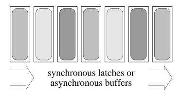
Figure 3.2: Synchronous or asynchronous block-aligned datapath communication
