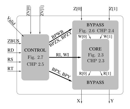
Figure 2.2: Schematic of the Register File process decomposition.
