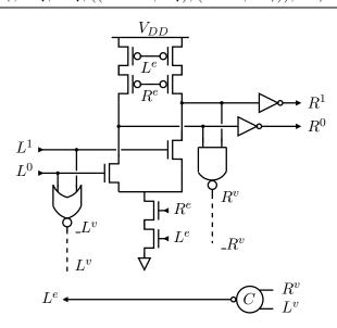
Figure 1.2: Precharge half-buffer (PCHB) with active-low acknowledgments
