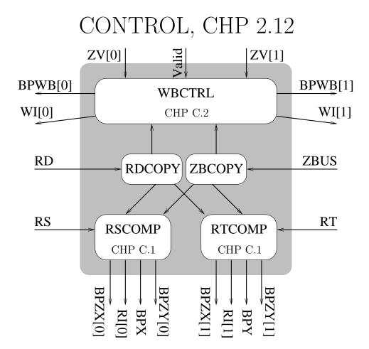
Figure 2.7: Schematic of the control decomposition
