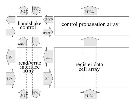
Figure 4.8: Floor decomposition of a write port block, shown with channel signals and some internal signals at component boundaries
