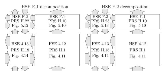
Figure 5.4: Floor decomposition of a PCEVFB WAD read port
